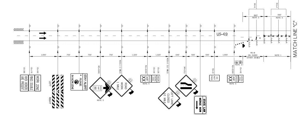
MAXIMUM SPACING BETWEEN CHANNELIZING DEVICES (FEET) SHALL BE TWICE THE POSTED SPEED LIMIT (M.P.H.) WITH THE FOLLOWING EXCEPTIONS, SPACING SHALL NOT EXCEED 50 FEET FOR CONES OR TUBE CHANNELIZERS. SPACING SHALL NOT EXCEED 75 FEET FOR CHANNELIZER CONES.SPACING SHALL NOT EXCEED 100 FEET FOR TYPE II BARRICADES, VERTICAL PANELS
